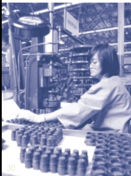
Machine operator inserts insulators into connectors, another of Avnet's value-added services.
